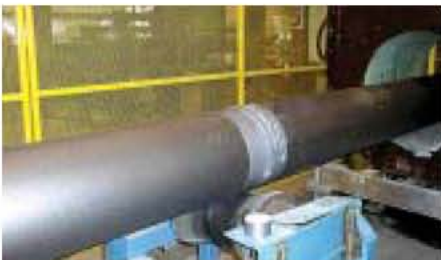
Sealing and Joining Fig.034 3M's line of Vinyl and Cloth Duct Tapes can be used in a variety of ways, including temporary sealing and joining pipe ends through a coating process.
