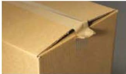
Tape Application Issues Fig.148
